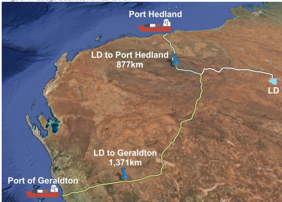
Existing Project studies have assumed SOP will be hauled by road train to the Great Northern Highway via the upgraded Talawana Track and then continue north to Port Hedland for shipping. An estimated haulage cost of \$104 per tonne of SOP was assumed, equivalent to 30% of the FOB operating cost estimate (refer to ASX Announcement dated 2 April 2015)<sup>1</sup>.
