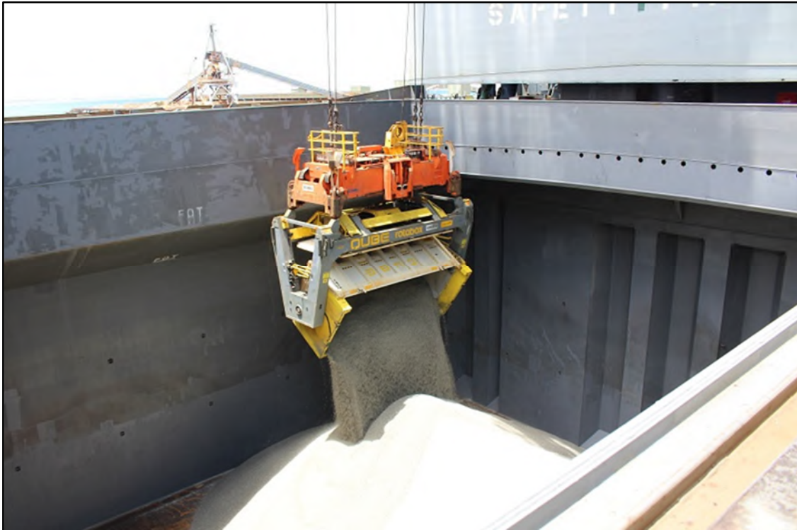
Figure 11b. Qube Rotabox Container being tipped into a shipping vessel
