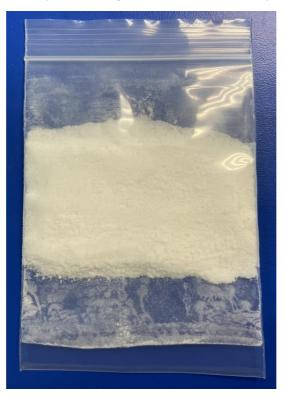
Earlier testwork conducted on the KP Lake Resource brine indicated that following evaporation of Resource brine to K saturation point of (ca. 45g/l K) treatment with Gypsum via the Reward Process method provided a first pass K recovery to Syngenite product of around 40%. Importantly, the 40% recovery figure for brines of composition similar to that of the KP Lake Resource brine, is possible without redissolution of precrystallised salts.
