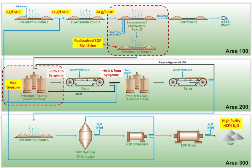
Figure 3 – Schematic Flowsheet for the Reward SOP Process.
