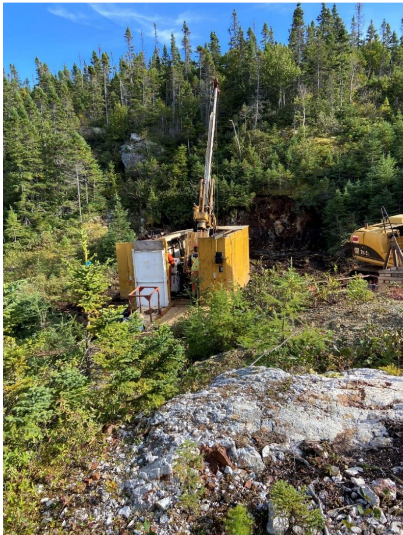
Figure 1 – Recent photograph of Reward's contracted diamond drilling rig positioned at the collar of the program's first diamond drill hole at the Jackpot Gold-Copper Prospect. The hole is testing for shallow, below-surface extensions of the mineralized Jackpot shear zone and quartz vein which is visible in the foreground.
